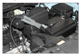
1. Set up the ammeter and voltmeter as shown in the figure.
